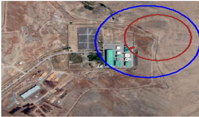
Figure 4. The release profile of \text{Cl}_2 gas from the catastrophic rupture scenario on PHAST software
